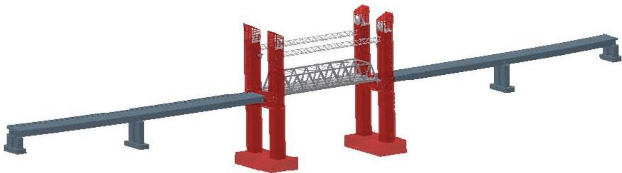
Figure 3. 3D drawing of lifting- and approach bridges
